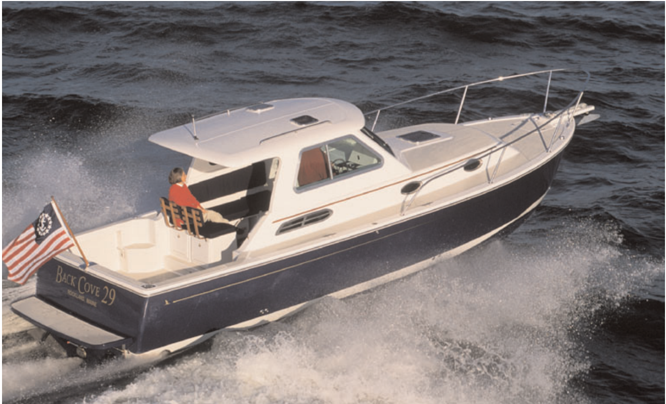
HIGH AND DRY: A stout pilothouse with tall windows and an overhang protect the owner and crew of the Back Cove 29 on a blustery day.
