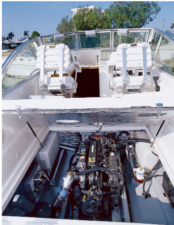
WHAT LIES BENEATH: A lift-up hatch provides access to the Yanmar diesel.
