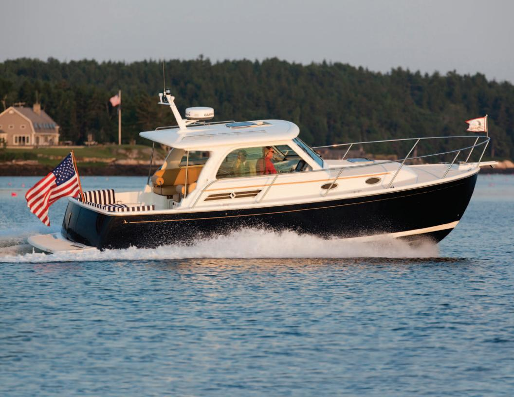
The Back Cove 30 is a fuel efficient single diesel engine/bow thruster combination. New diesels of the type installed in the Back Cove 30 employ modern fuel injection technologies, are cleaner running and far quieter. Cruise speeds with her standard 315 hp engine are in the 20 knot range, and optional engines are available that will raise cruise speeds to the mid-twenties.
