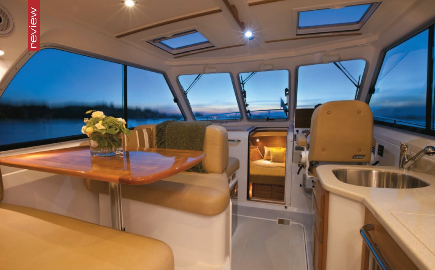
TOP: THE HELM DECK IS AIRY AND BRIGHT, WITH OVERHEAD HATCHES, OPENING SIDE WINDOWS AND A CENTRE-OPENING WINDSHIELD.
