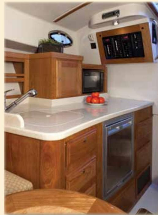
Aft and to starboard is the galley, a functional space with solid surface countertop, stainless steel sink, alcohol/ electric stove, microwave oven and AC/DC fridge. There are many drawers and lockers for storage. Opposite to port, a full molded head compartment has a fresh water electric flush MSD, a solid surface countertop and pull out shower faucet.
