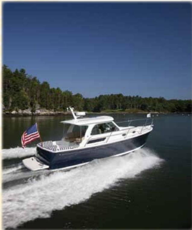
The Back Cove 30 is a fuel efficient single diesel engine/bow thruster combination. New diesels of the type installed in the Back Cove 30 employ modern fuel injection technologies, are cleaner running and far quieter. Cruise speeds with her standard 315 hp engine are in the 20 knot range, and optional engines are available that will raise cruise speeds to the mid-twenties.
